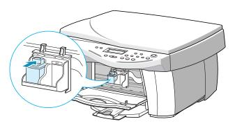
**6** Unwrap and remove the black print cartridge from its plastic bag. Holding the cartridge at the top, carefully remove the sealing tape covering the print head.
